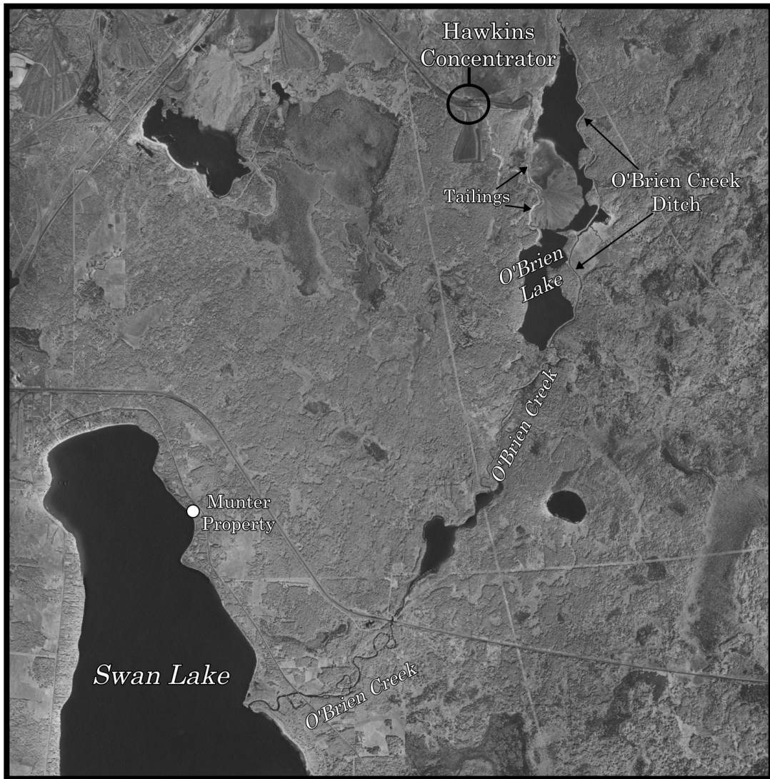
Figure 5.5: Aerial image of the Hawkins concentrator from 1947, showing O'Brien Creek Ditch, Munter's property, and spread of tailings (Adapted from Minnesota DNR Airphotos Online)
